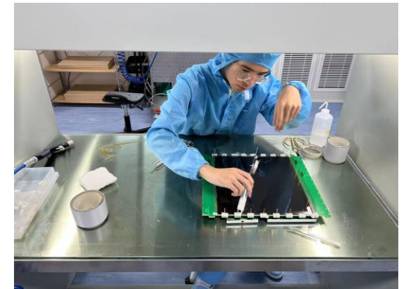
Use fishing line to create gas gaps
