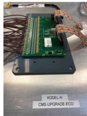
iRPC prototype opened and KODEL electronics
