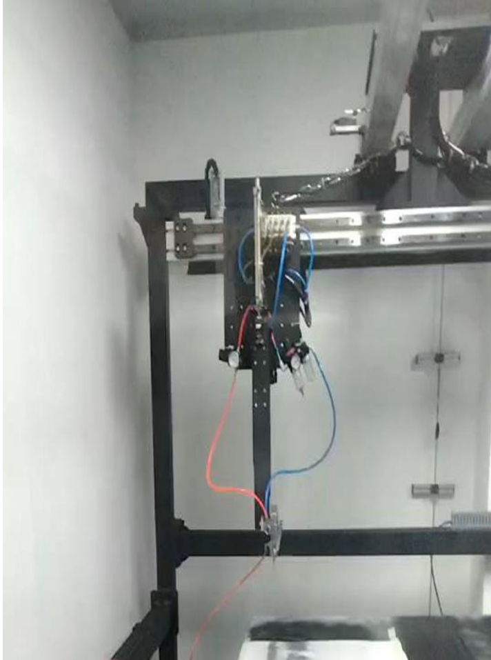
Graphite spraying system: A spray gun held on a 2-D gantry
