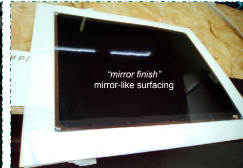
HPL electrode after lamination
