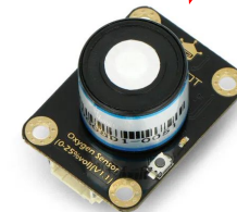
Oxygen sensor (model: SEN0322)
