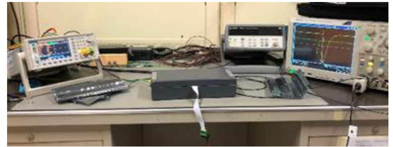
FE boards testing @CERN BB5
