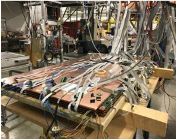
Efficiency measurements of individual detectors before integration @BB5
