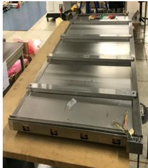
Fully integrated RPC doublet
