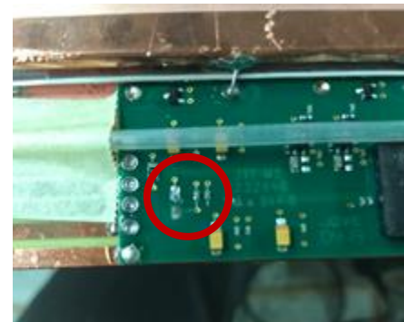
Replacing FE board/s to fix dead channels
