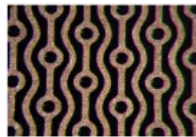
Figure 2. A single-phase TPC with a L-MHSP (or L-COBRA, shown) coated underneath with CsI. Ionization electrons and UV-induced photoelectrons from CsI are collected into the L-MHSP holes, and drift towards the anode strips. VUV photons emitted by EL + small avalanche near the strips, are detected by the top photo-sensors. Another fraction of S1 photons are detected by bottom photo-sensors.
