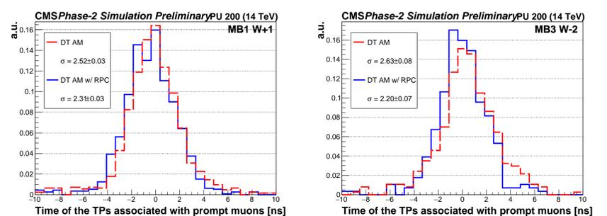
Figure 2: LEFT: The timing distribution of the trigger primitives associated with a generated muon with DT AM (Analytical Method) (Red line) and DT AM + RPC (Blue line) for the station 1 and wheel +1 (MB1 W+1). RIGHT: The timing distribution of the trigger primitives associated with a generated muon with DT AM and DT AM + RPC for the station 3 and wheel -2 (MB3 W-2).
