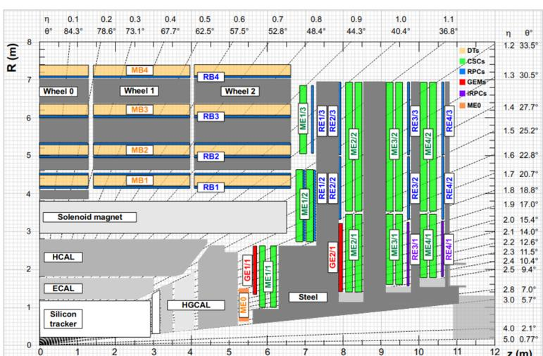
Figure 1: Schematic longitudinal view of one quarter of the CMS detector with the different subsystems which compose the Muon Detector for the Phase-II upgrade of LHC [1].
