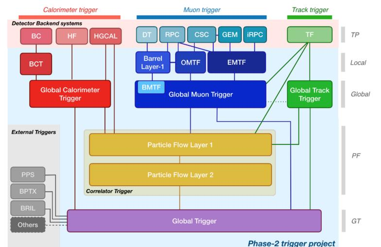
Functional diagram of the CMS L1 Phase-2 upgraded trigger design [2].
