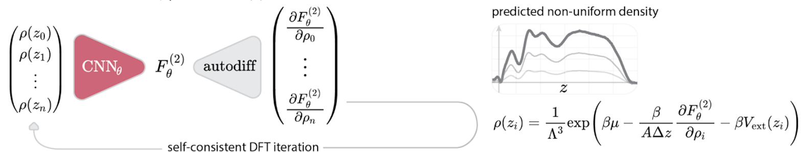
FIG. 1: 1. Bulk densities in planar geometry \rho(z_i) = \rho_b and radial distribution functions g(r) are sampled from Monte Carlo simulations of homogeneous bulk systems of Lennard-Jones particles. Each g(r) is converted to the second functional derivative of the excess free-energy \delta^2 \mathcal{F}_{\text{exc}} / \delta\rho(z_i)\delta\rho(z_j) by employing the Ornstein-Zernike equation. 2. Through automatic differentiation (autodiff 2 ), the neural functional F_\theta^{(2)} is optimized to fit the Hessian of the model output with respect to input density profiles to \delta^2 \mathcal{F}_{\text{exc}} / \delta\rho(z_i)\delta\rho(z_j) . 3. The optimized model can then be applied in cDFT to obtain non-uniform equilibrium density profiles through automatic differentiation (autodiff) and the free energy F_\theta^{(2)} for a system of Lennard-Jones particles subjected to arbitrary external potentials.
