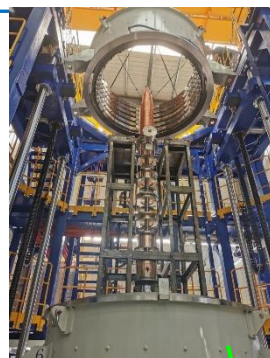
Klystron No. 2 aiming at efficiency 77%
