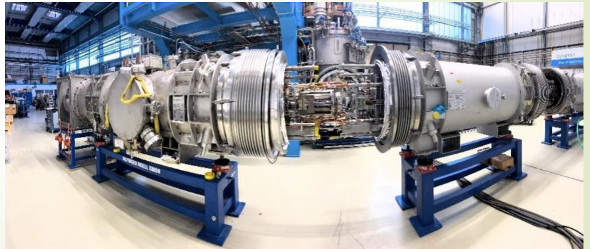
First thermal cycle of the SIS100 string
