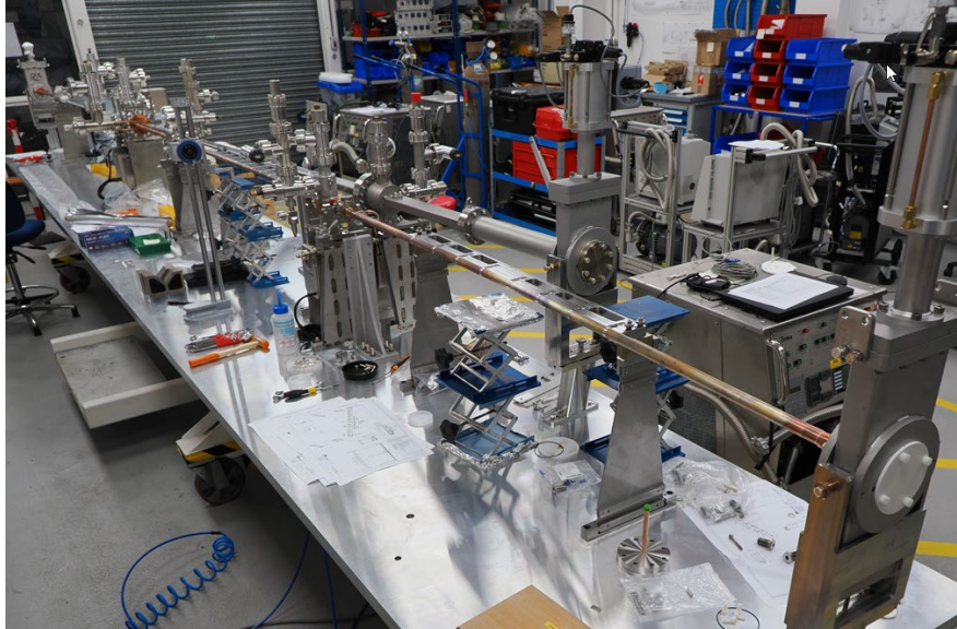
Complete LM vacuum string assembly (Al LM VC2)
