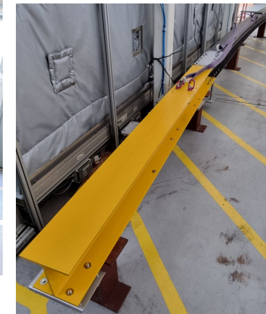
Trial lifting beam
