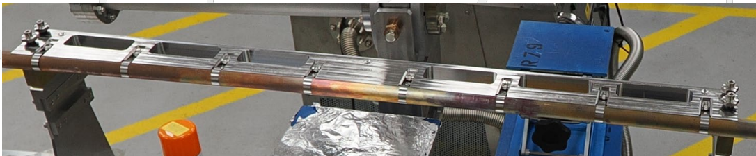
Complete LM vacuum string assembly (Al LM VC2)
