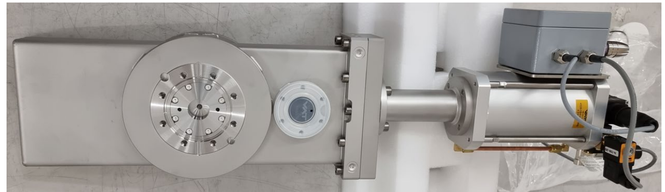
Gate valve with internal RF shield
