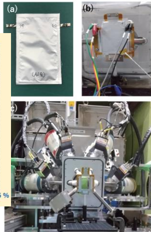
Figure 1. (a) A Li-ion battery sample. (b) The sample set from aluminum holder at the ISIS MIXE. The detector detectors and Si drift detectors from the downstream the main beam at the D2 experimental area.
