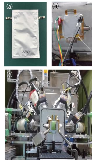
Figure 1. Pictures of (a) a Li-ion battery sample, (b) the sample set in an aluminum holder at the measurement position with cables, and (c) the sample holder and Ge semiconductor detectors and Si drift detectors from the downstream of the muon beam at the D2 experimental area.
