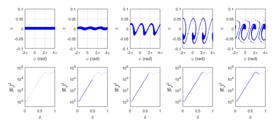
The evolution consists of several stages; an initial start-up (lethargy) phase, exponential growth, followed by saturation. The height of the FEL bucket can be seen to grow along the length of the undulator.
