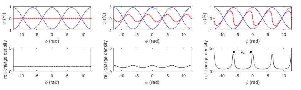
As the electrons start to change energy and rotate in the FEL bucket, the electrons that gain energy move forward in phase, and those that lose energy move backwards. The electrons will bunch together at the synchronous phase, and micro-bunches will start to form at the radiation wavelength and begin to emit coherently.
