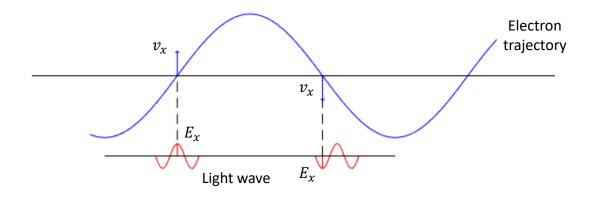
This is the same condition as for constructive interference in an undulator, i.e. the condition for continuous energy transfer from the electron beam to the light wave is:
