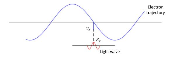
As the electrons travel along the undulator, the radiation slips forward ahead of the electrons. In order for there to be sustained energy transfer from the electron beam to the light wave, the light wave must advance by  $\lambda_r/2$  when the electrons have travelled a distance  $\lambda_u/2$ .
