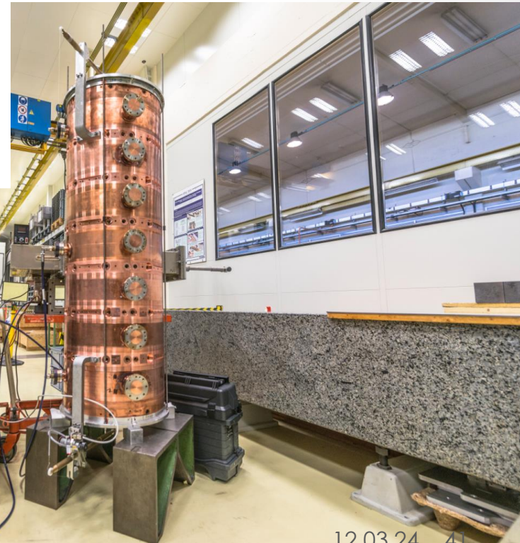
Figure 1: 3D-view of the full prototype PIMS cavity.
