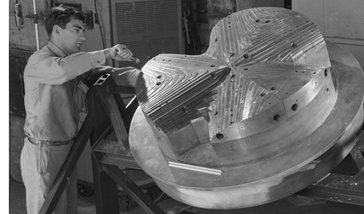
AVF concept – harmonic pole shaping, electron model, Richardson et al (1950), courtesy of Lawrence Berkeley National Laboratory
