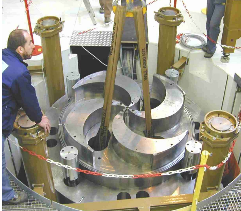
PSI/Varian comet: 250MeV sc. medical cyclotron
