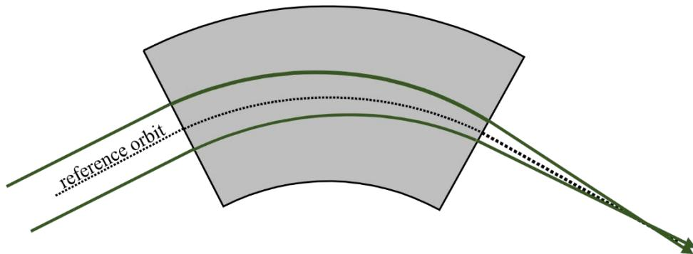
*Transversely displaced beam
