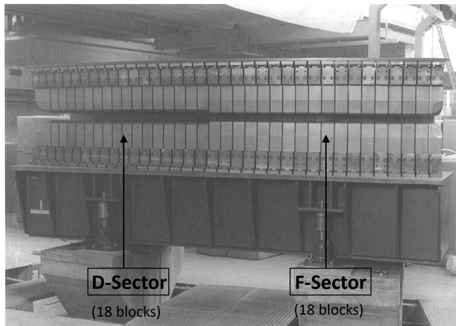
Nowadays: Alternating gradient focusing with strong focusing quadrupoles.
