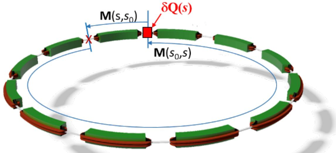
A gradient error will not influence the closed orbit but the betatron function of the lattice. In order to calculate the betatron amplitude modulation, we have to determine the single turn transport matrix starting at a given observer position  $s$ , introducing a small gradient perturbation at position  $s_0$
