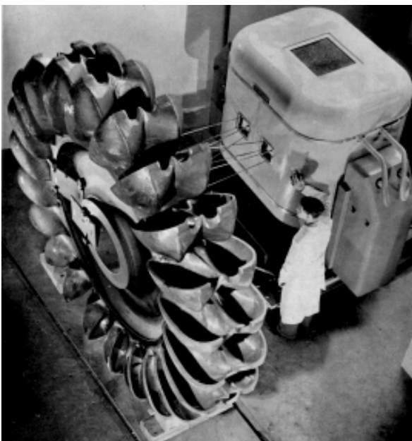
Fig. 10.6: A beta-tron being used to test a Pelton-wheel at Georg Fischer AG, Schaffhausen (photograph: BBC).
