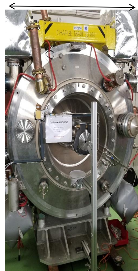
Accelerating Cavity, freq = 80 MHz (CERN PS) All pictures © CERN
