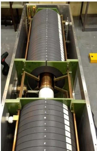
Ferrite Loaded Cavity, freq = 3 – 8 MHz (CERN PS Booster)
