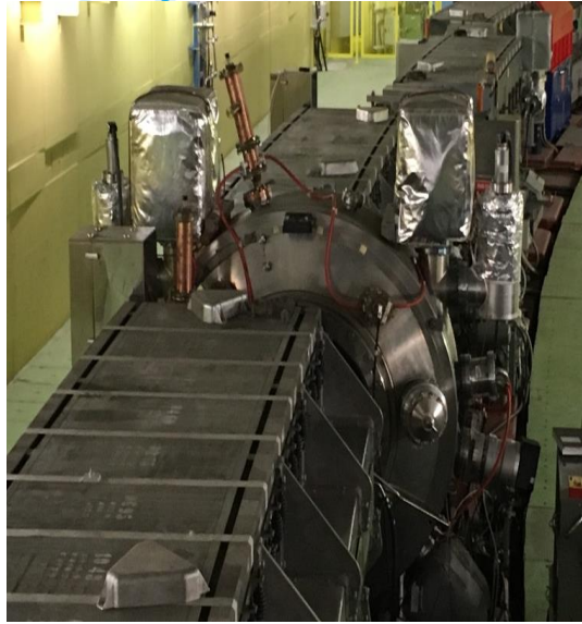
PS single cell cavity ("pillbox")
