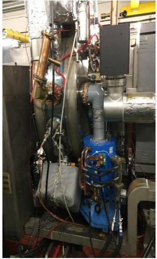
PS single cell cavity ("pillbox")
