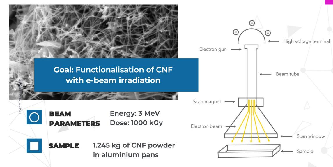
iFAS Linear accelerator commercially available through IONISOS (France)
