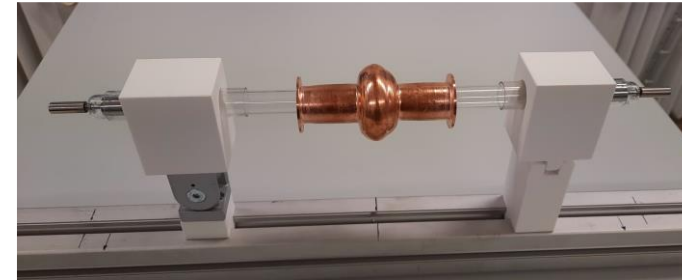
Holding system for the flash lamp and cavity
