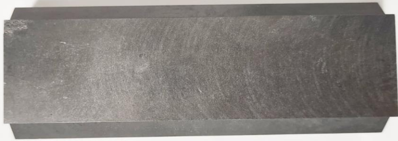
CrGr block, machined in the shape of HL-LHC collimator absorber
