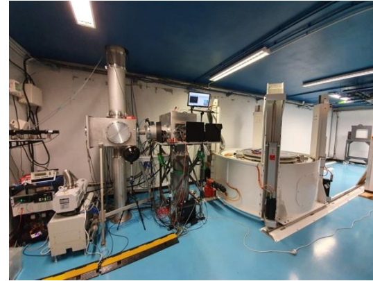
KAIO-based NDT platform with a 10 Hz Ti:Sa laser (SHERIL platform at LOA)
