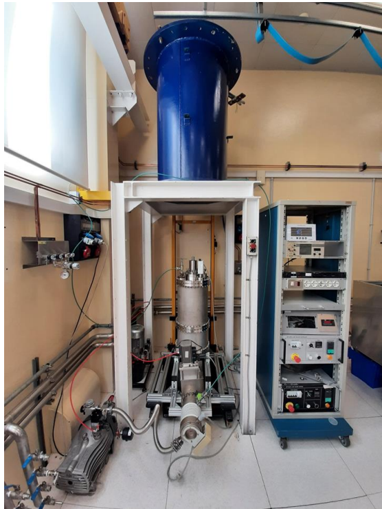
PVD Coating facilities for planar samples and 1.3 GHz cavities
