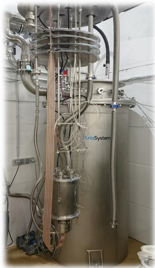
Bath cryostat for vertical cavity testing
