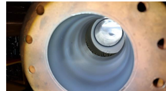
Coated 1.3 GHz Dummy Cavity
