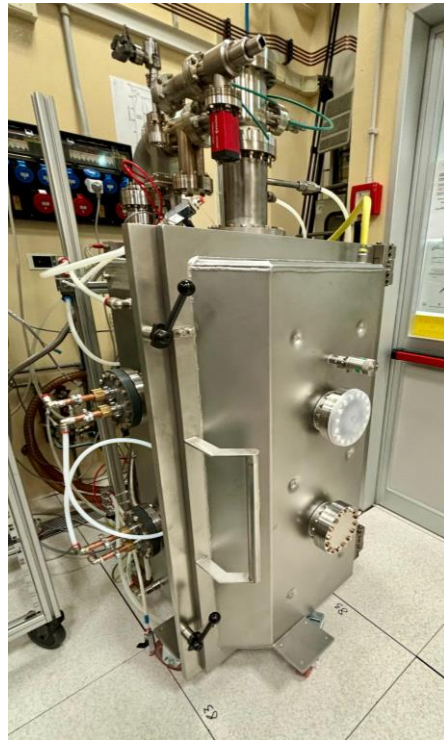
PVD Coating facilities for planar samples and 1.3 GHz cavities
