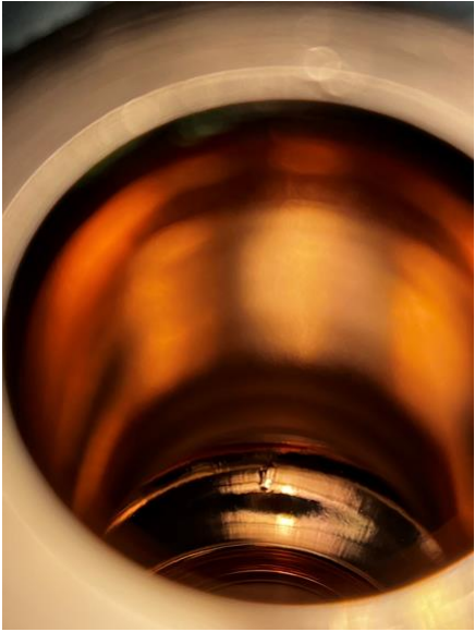
6GHz cavity EP polished
