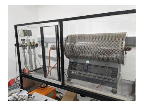
Alongside film deposition. A tube furnace was recommissioned for post annealing.
