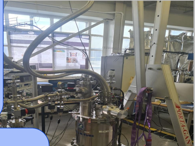
Magnetic Field Penetration Insert (EXP 800).
