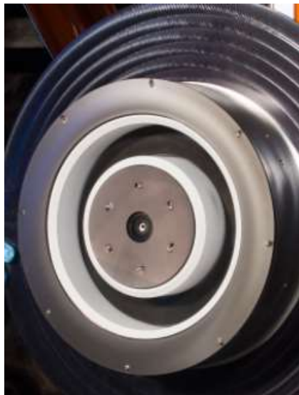
Picture courtesy of Nasa. HERMeS: NASA's SPT Thruster. Inner and outer wall of BN composite.
