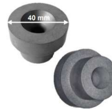
Subscale nozzles machined after sintering. Both EDM and conventional machining are possible.
