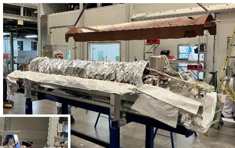
Cold mass being equipped with magnetic & thermal shield
