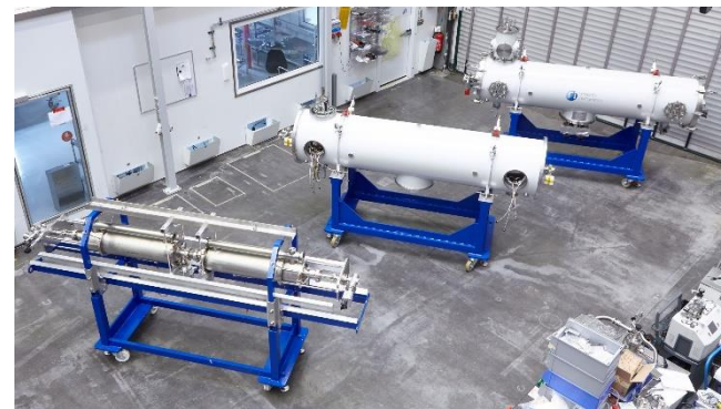
Cold mass being equipped with magnetic & thermal shield
