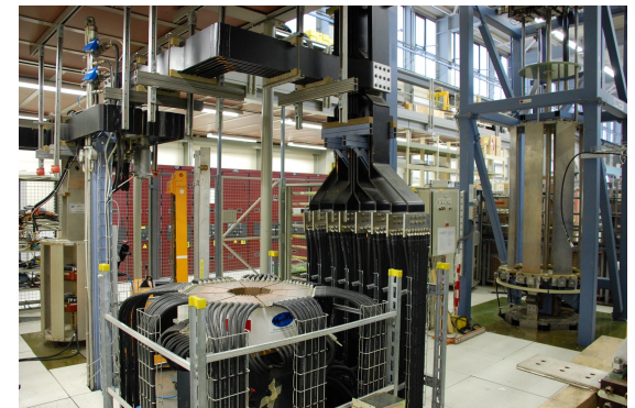
20 kA DCCT test bed
