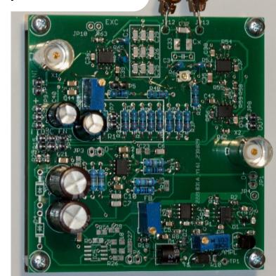
We are modelling input circuitry, striving for lower noise and lover drift then 3458A, while also characterising performance of the latest JFET matched pair transistors
