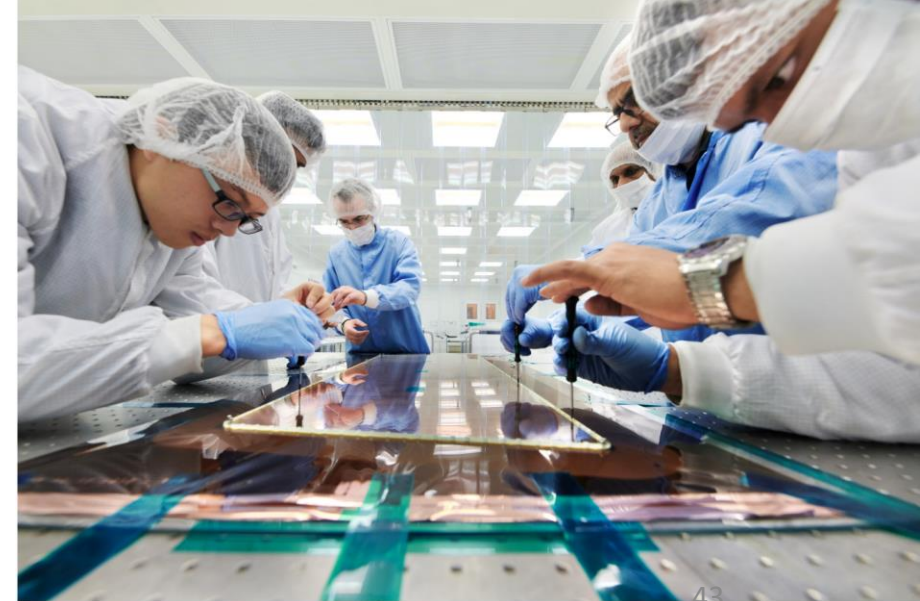
Assembly of the GEM detectors at CERN in clean room (Image: CERN)
