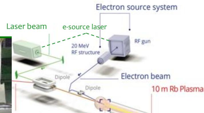
A Photo-injector originally built for a CLIC test facility is now used as electron source for AWAKE producing **short electron bunches at an energy of ~20 MeV/c.**
