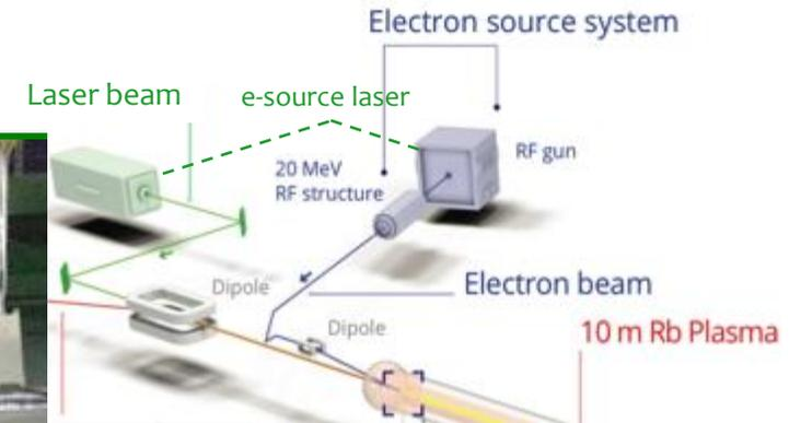
A Photo-injector originally built for a CLIC test facility is now used as electron source for AWAKE producing **short electron bunches at an energy of  $\sim 20$  MeV/c.**
