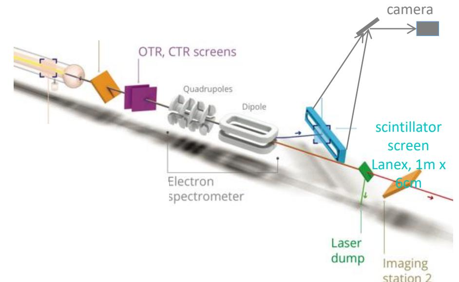
Electrons will be accelerated in the plasma. To measure the energy the electrons pass through a **dipole spectrometer** and the dispersed electron impact on the **scintillator screen**. The resulting light is collected with an intensified CCD camera.
