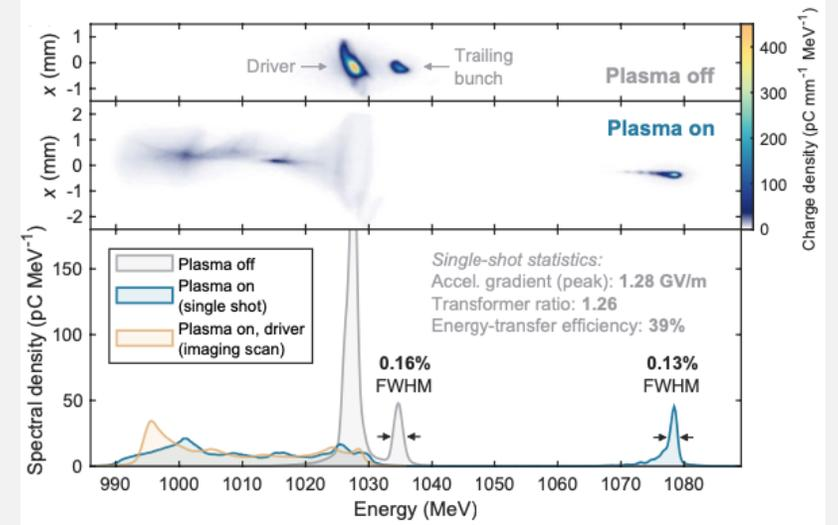
Transfer efficiency **42+/-4%** with **0.2% energy spread**, Up to **70%** when allowing energy spread increase
