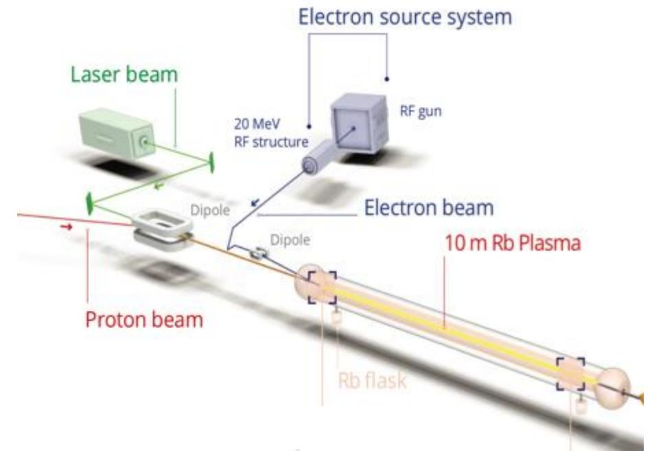
The AWAKE beamline is designed to deliver a **high-quality beam** to the experiment. The proton beam must be steered around a mirror which **couples a terawatt class laser** into the beamline. Further downstream, the **witness electron beam** will be injected into the same beamline.
