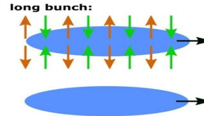
The experiment induces a plasma instability, this instability modulates the long proton beam into a sequence of short beams (micro-bunches). These micro-bunches resonantly drive high wakefields!  $\rightarrow$  **immediate use of SPS proton bunch!**
