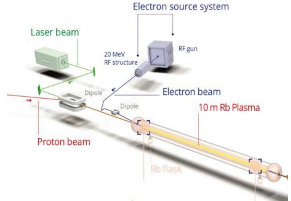
The AWAKE beamline is designed to deliver a **high-quality beam** to the experiment. The proton beam must be steered around a mirror which **couple a terawatt class laser** into the beamline.
