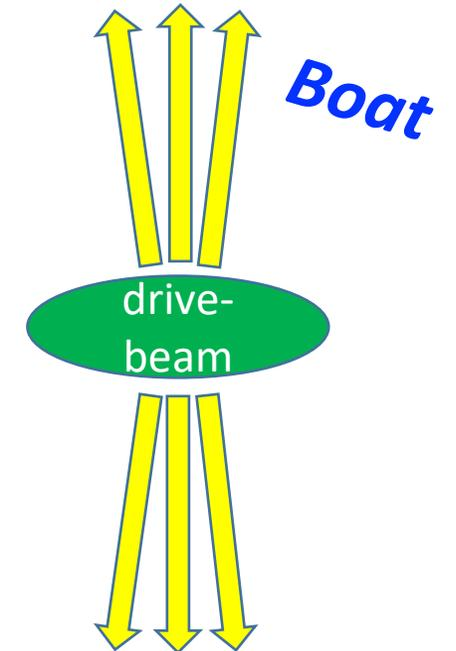
Using plasma to convert **the transverse electric field** of the drive bunch into a **longitudinal electric field in the plasma**. The more energy is available, the longer (distance-wise) these plasma wakefields can be driven.
