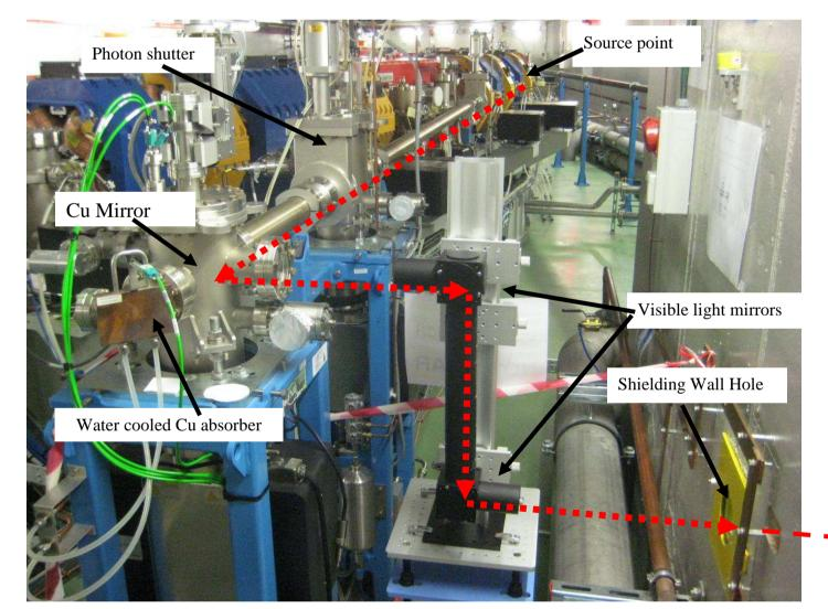
In-vacuum mirror reflects just the visible part of the synchrotron radiation. 6 in-air commercial mirrors direct the light from the inside to outside the tunnel (Di. Hutch).
