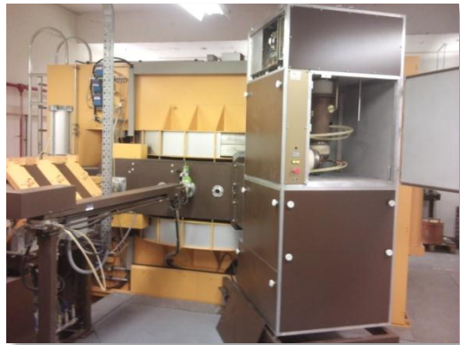
Fig. 6. Scanditronix MC-60 cyclotron is an isochronous machine. Magnetic field corrects the relativistic mass effect: m = \gamma \cdot m_0 , to hold the synchronism
