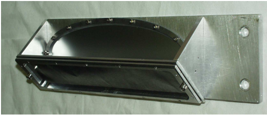
FIG. 6. A support for a 150\text{ mm} \times 50\text{ mm} surface area and 50\ \mu\text{m} thick spectrometer screen with a carbon foil in front for blocking synchrotron radiation.
