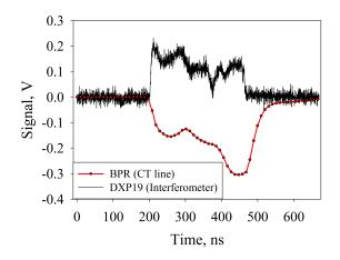
FIG. 14. Signals from the DXP19 detector in the interferometer and the RF-pickup in the Transfer Line 1.
