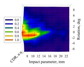
FIG. 8. Vertical polarisation of the CDR distribution measured by DXP15 detector. The targets impact parameters h1=27mm; h2=7mm.
