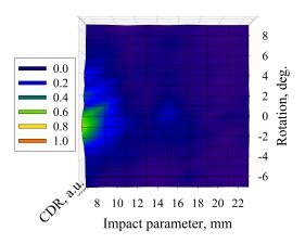
FIG. 9. Vertical polarisation of the CDR distribution measured by DXP15 detector. The targets impact parameters h1=7mm; h2=7mm.
