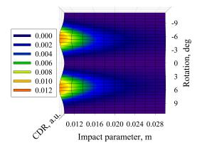
FIG. 5. Horizontal polarisation of the CDR distribution. The targets impact parameters h1=10mm; h2=10mm.
