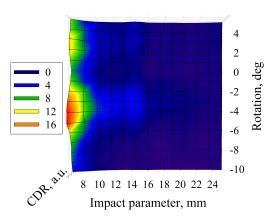
FIG. 11. Horizontal polarisation of the CDR distribution measured by DXP15 detector. The targets impact parameters h1=7mm; h2=7mm.
