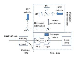
FIG. 7. Schematic layout of the CDR experiment.
