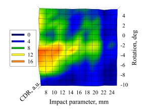
FIG. 10. Horizontal polarisation of the CDR distribution measured by DXP15 detector. The targets impact parameters h1=30mm; h2=7mm.
