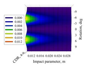
FIG. 4. Horizontal polarisation of the CDR distribution. The targets impact parameters h1=30 mm; h2=10 mm.
