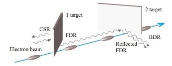
FIG. 1. Schematic layout of the Dual Target System at CTF3. FDR - Forward Diffraction Radiation; BDR - Backward Diffraction Radiation; CSR - Coherent Synchrotron Radiation.
