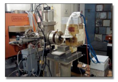
PMT gain and variable parameters of the electronics have been tuned to find the optimal <u>working point</u>. Mainly to avoid saturation fenomena (very high number of electrons expected) The BTF provides electron bunches, with a known variable total charge. Measuring the prototype detector signal vs the electron charge a <u>calibration curve</u> has been obtained
