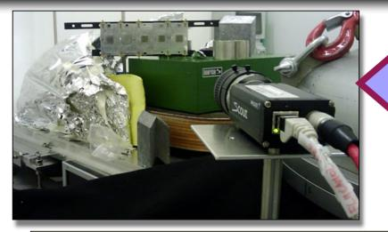
While commissioning the readout electronics, an alternative purely optical readout system has been realised: the light emitted by the scintillating fibers is recorded by **CCD cameras**.
