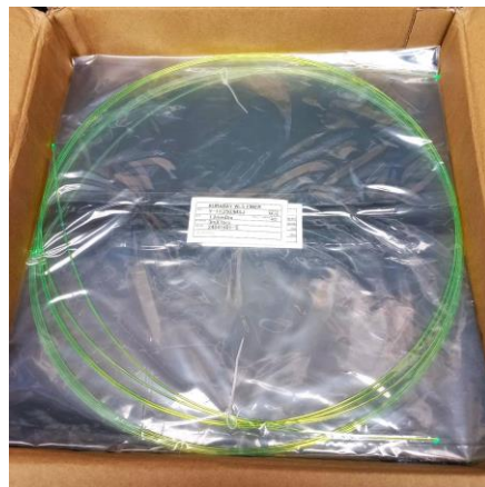
Kuraray Wavelength Shifting (WLS) Fiber
