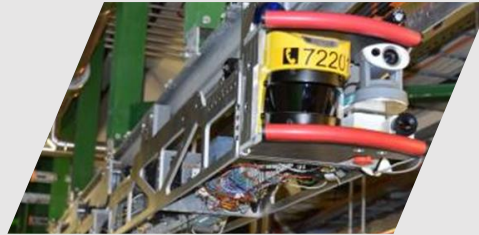
CERN Tunnel Inspection Monorail (TIM)
