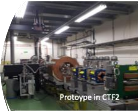
S-band e-gun (INFN) with X-band accelerator (CLIC/CLEAR)
