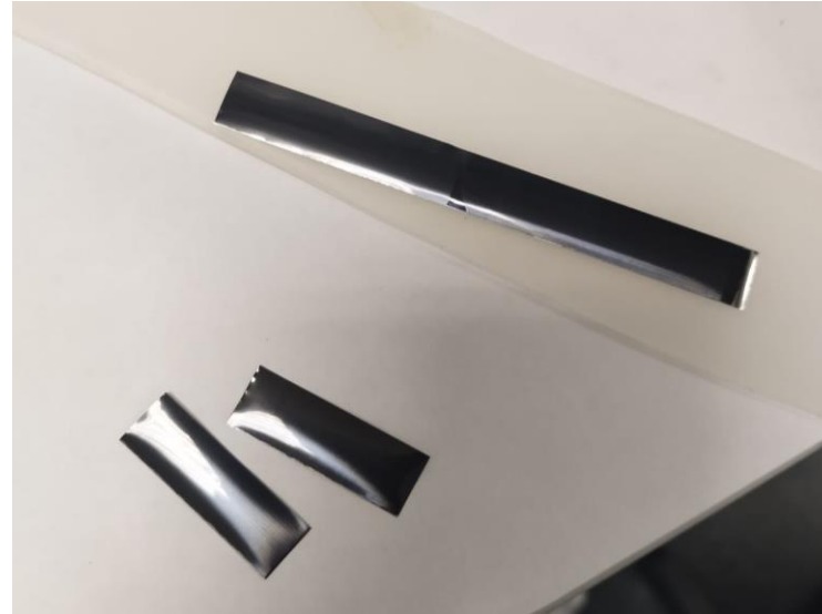
2 nd – Transfer to 20 \mu\text{m} thick low-RF loss Kapton ( <1 dB/m loss @6 GHz)
