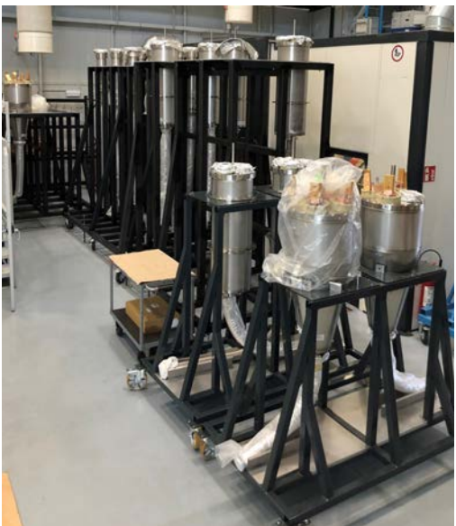
Assembly and storage of cryostats
