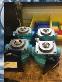
Revision of STAL pumps
