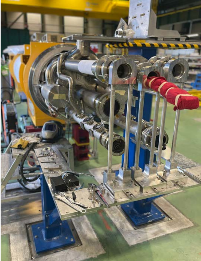
Corrector package assembled in SMI2. Magnet ready to be tested.
