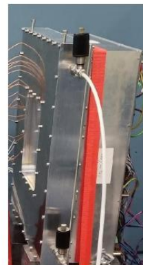
Front: Aluminium entrance window (0.2 mm thick)
