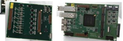
Back: Front End Electronics and triggering boards (custom)
