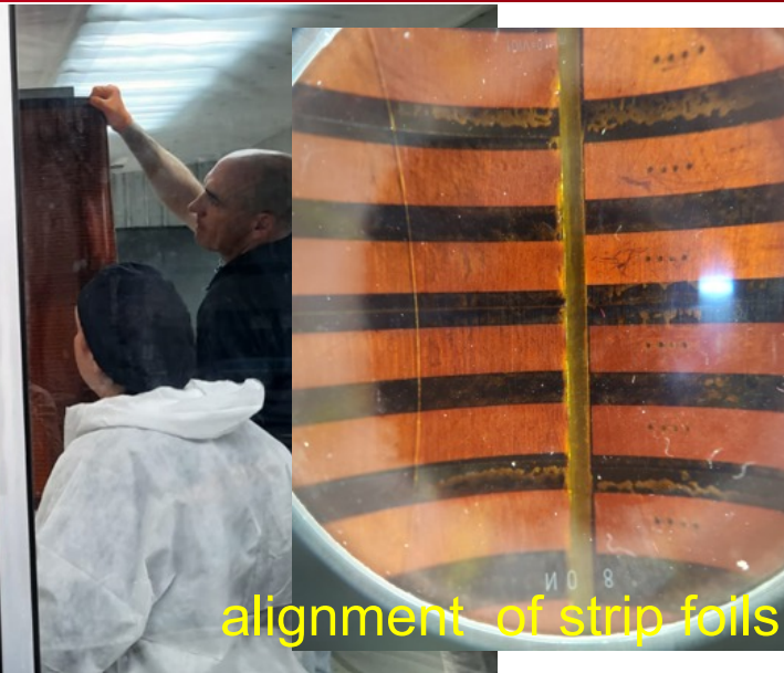
Lamination of New kapton layer
