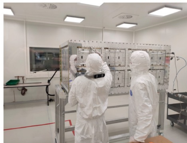
Leak test after ERAM installation
