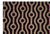
Figure 2. A single-phase TPC with a L-MHSP (or L-COBRA, shown) coated underneath with CsI. Ionization electrons and UV-induced photoelectrons from CsI are collected into the L-MHSP holes, and drift towards the anode strips. VUV photons emitted by EL + small avalanche near the strips, are detected by the top photo-sensors. Another fraction of S1 photons are detected by bottom photo-sensors.
