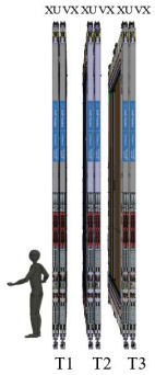
Scintillator Fibres The front and profile view of detector planes JINST 19 (2024) 05, P05065
