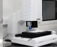
MICRO-VU Vertex 261 Programmable 3D measuring system
