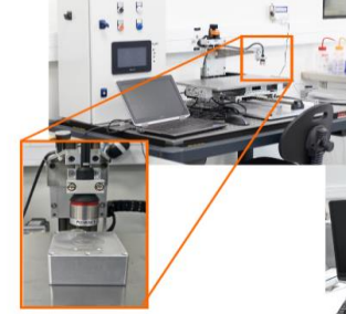
KEYENCE CL-3000 + CL-P015 Confocal Profilometer (res. 0.15 µm)
