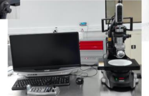
KEYENCE VHX-7000 High-resolution digital microscope (20x → 2000x)
