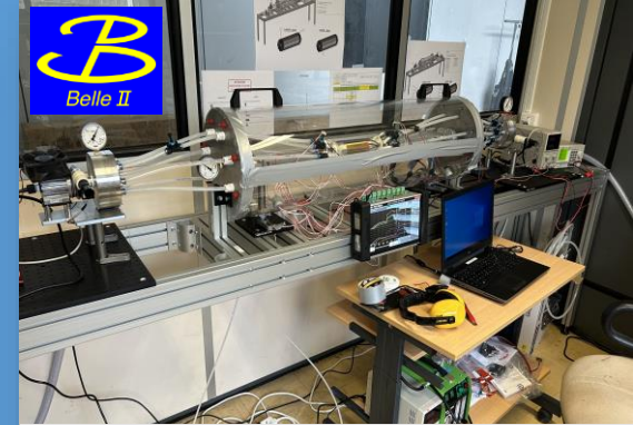
Inner vertex detector air cooling test bench for Belle 2 upgrade
